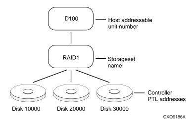
Figure 3–13. Locating Devices using PTLs
